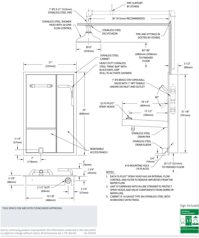
**GBF2152** Recessed Safety Station with Drain Pan and Daylight Drain, Exposed Shower Head
