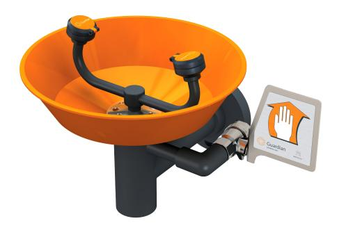
**Application:** Eyewash for wall mounting. Unit is constructed of PVC, PVC-coated components and a stainless steel valve for superior corrosion resistance. Ideal for industrial environments where harsh acids and caustics are present. Two GS-Plus™ spray-type outlet heads deliver a flood of water for rinsing eyes.
