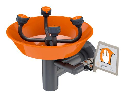
**Application:** WideArea<sup>™</sup> eye/face wash for wall mounting. Unit is constructed of PVC, PVC-coated components and a stainless steel valve for superior corrosion resistance. Ideal for use in industrial environments where harsh acids or caustics are present. Four GS-Plus™ spray-type outlet heads deliver a flood of water over a wide area of coverage for complete rinsing of eyes and face.
