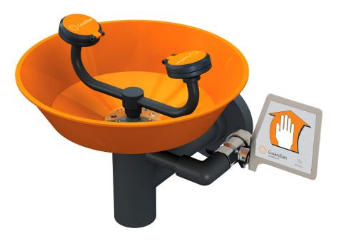
**Application:** Eye/face wash for wall mounting. Unit is constructed of PVC, PVC-coated components and a stainless steel valve for superior corrosion resistance. Ideal for use in industrial environments where harsh acids or caustics are present. Two large FS-Plus<sup>™</sup> spray-type outlet heads deliver a flood of water for rinsing eyes and face.
